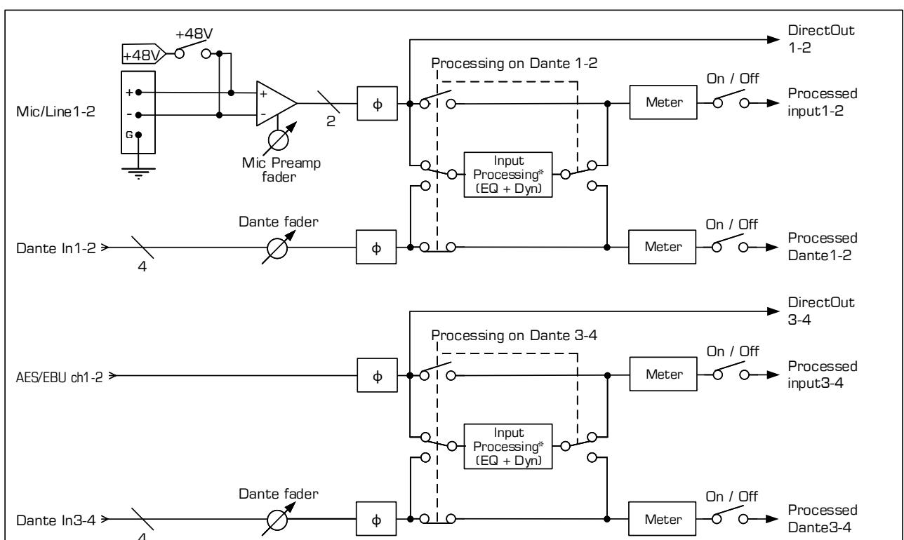
Diagram of the AVDT-BOB's Input Processing block for ADE8io/ADX8io
