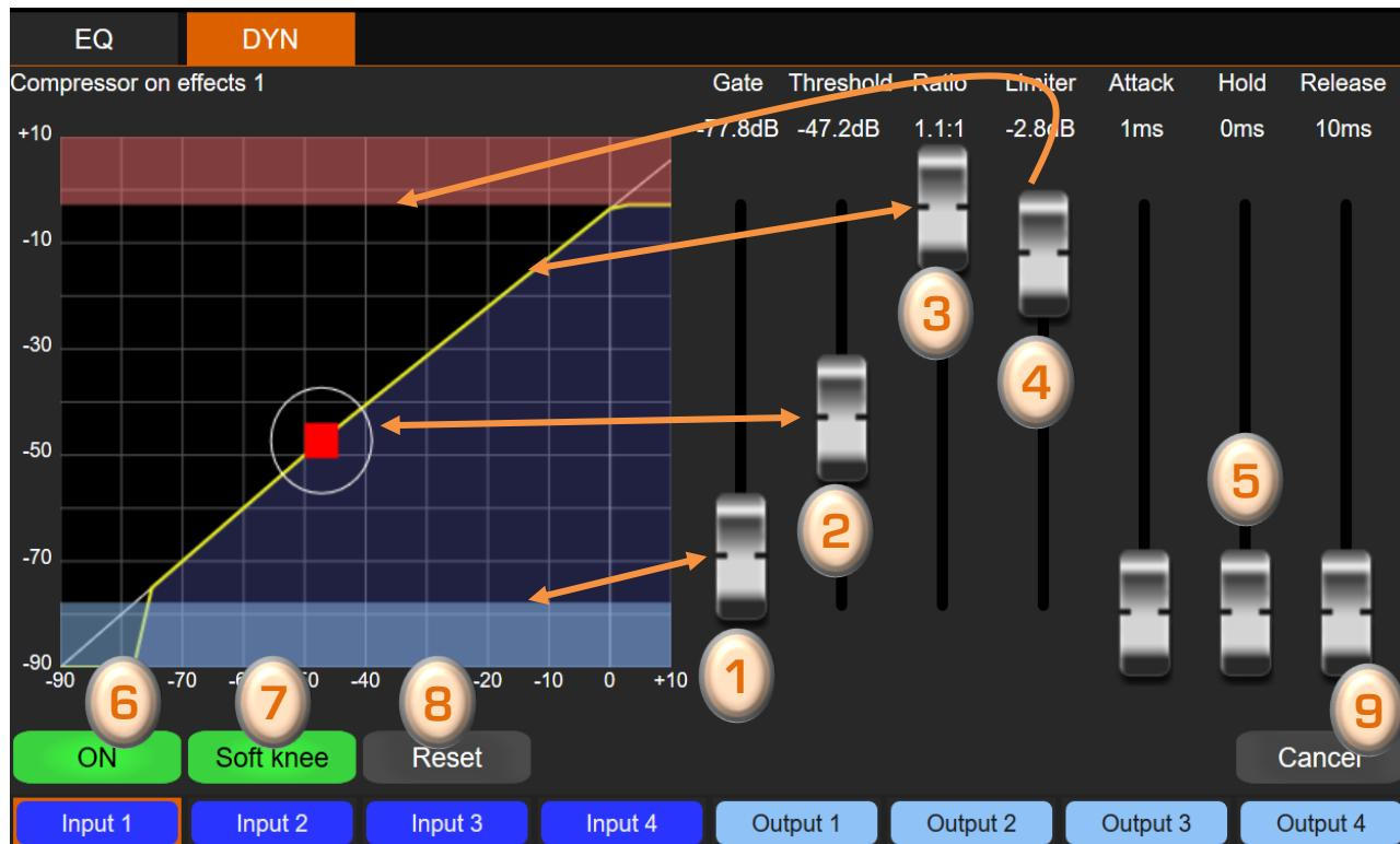
1. The first fader controls the Gate level of the processing (mutes the sound when the signal is too weak)
