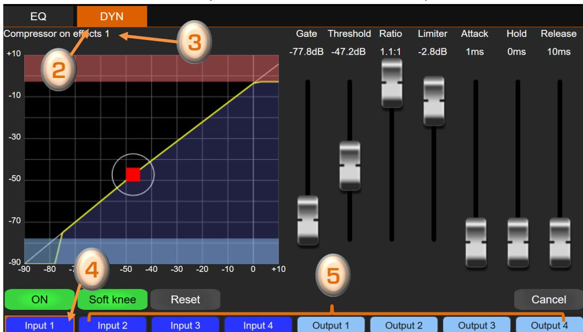
3. On the top left, a reminder indicates to which physical input/User's name the EQ/DYN processing is attached,
