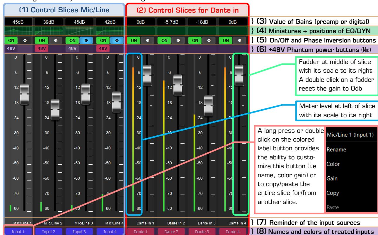
1. On left, 4{2} slices of faders and buttons control the Mic/Line preamps and processing
