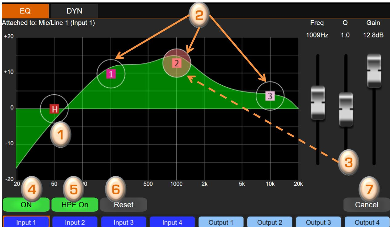
1. (H) button position manages the frequency parameter of the High pass filter
