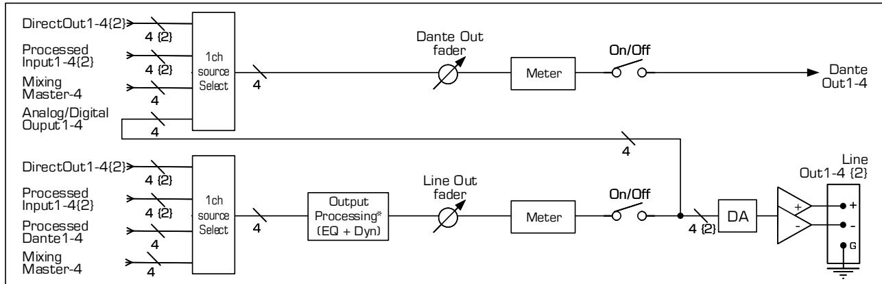
*Diagram of the AVDT-BOB's Output Processing block for AE4io/AE8io/AS8io versions*
