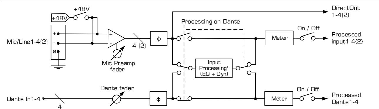
Diagram of the AVDT-BOB's Input Processing block for AE4io/AE8io/AEG6io/AS8io versions
