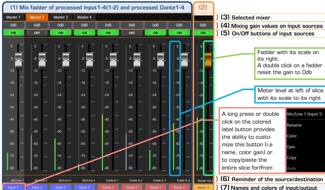
1. On left, 8{6} individual slices of faders and buttons control of the processed inputs from the input processing
