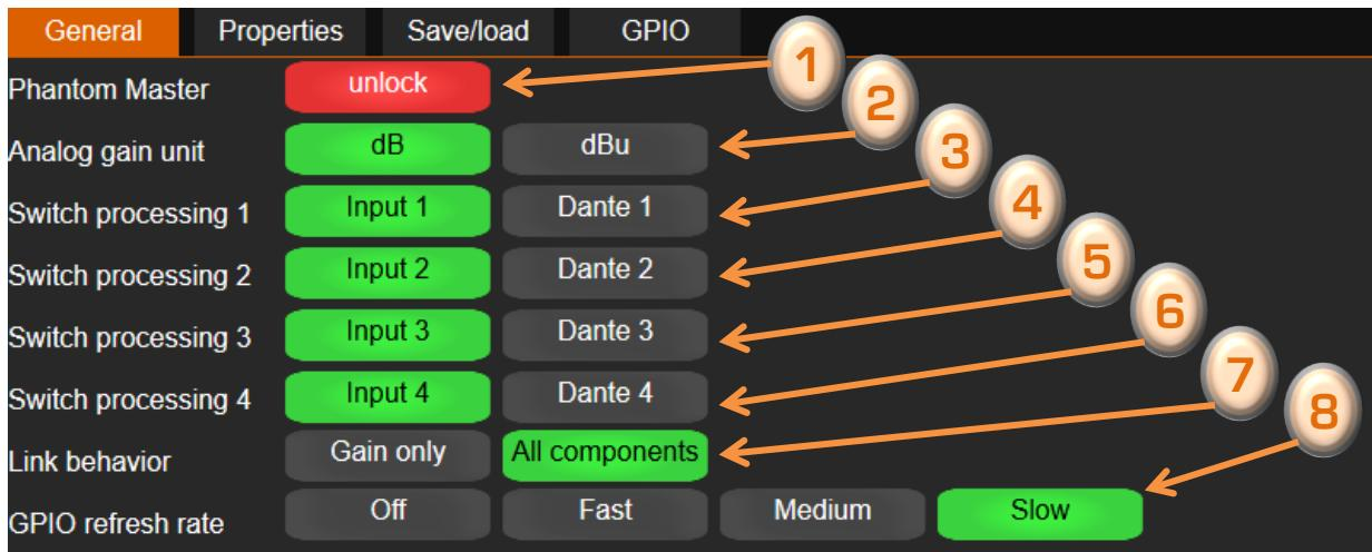
1. Phantom Master button locks/unlocks the +48V button of Mic/Line phantom power
